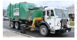
**Garbage truck, trash truck** ... These trucks have many names, but only one sole purpose. Most of ACES' residential fleet are side-loaders. A hydraulic arm on the right side of the truck grabs the trash or recycling cart from the curb and dumps it into the hopper opening ... the driver sits on the right side so he can make sure all the trash falls into the right place. These big trucks could make over 1,000 stops and hold up to 19,000 lbs. of trash per load!
