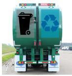
**Two trucks in one** ... You may have seen your driver dumping both the garbage and recycling at the same time, but not to worry! This nifty split body truck is designed specifically to pick up both commodities at the same time. When servicing the garbage, the driver simply pushes a button to block the recycle hopper and vice versa. The trash is dumped into one side of the truck and the recycling is dumped into the other. They are completely separate compartments!
